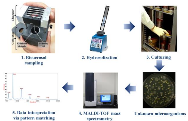
Figure 1. Processes of field test for indoor air monitoring.
